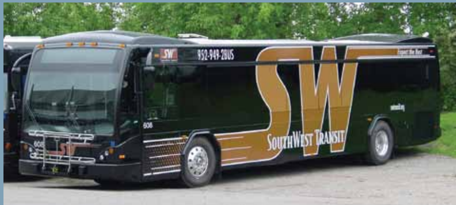
Left: 40-foot bus wrapped with a combination of digitally printed perforated vinyl window film, copper metallic vinyl film, and reflective vinyl letters; Middle: Ten-foot-high sign on Alupalite using a VUTEK PressVu UV 200/600 by EFI; Right: Signs created for Americinn Perk on 1/4-inch-thick white PVC Panels.
